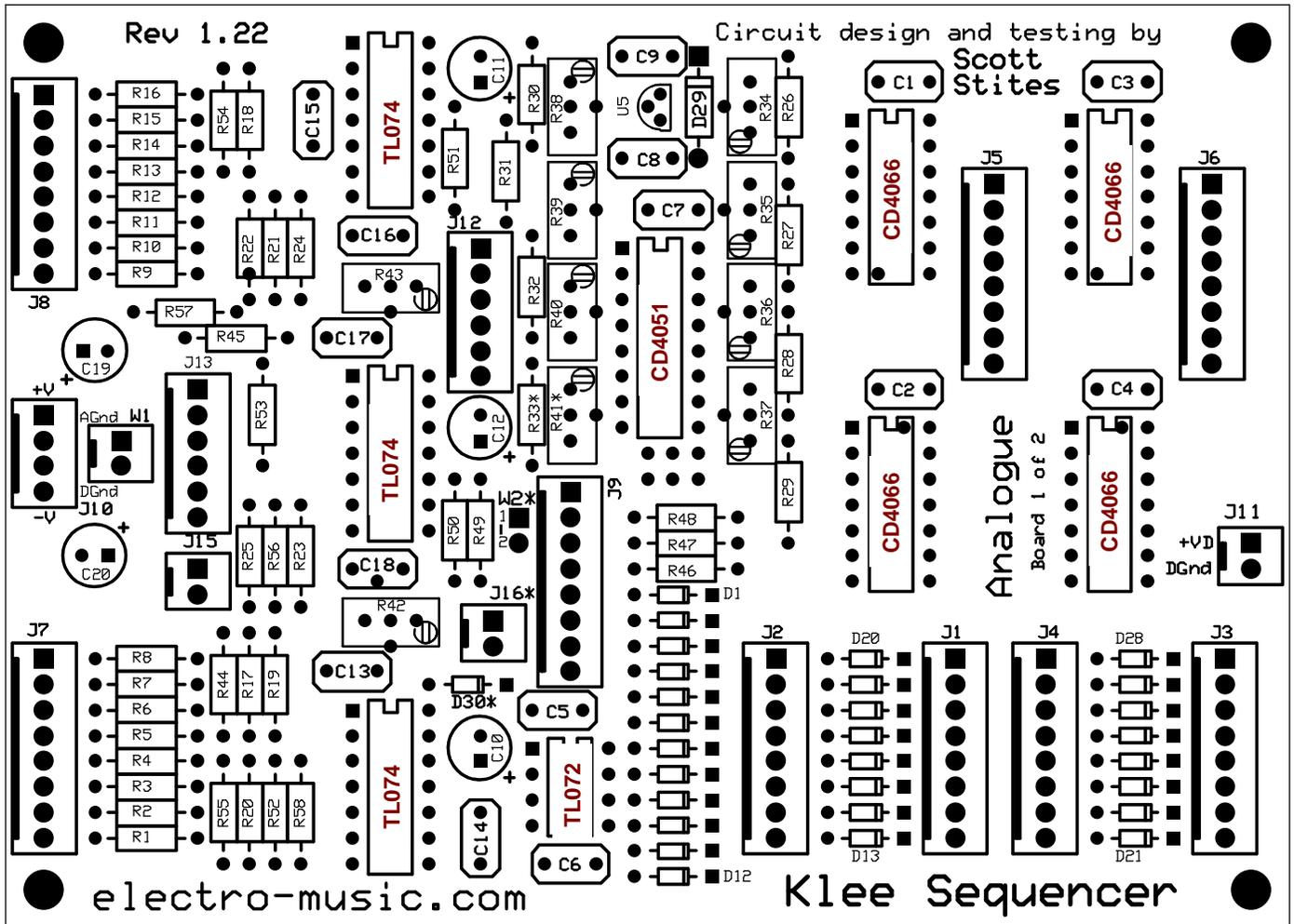
Figure 7-11: Analogue Board IC Placement Guide
