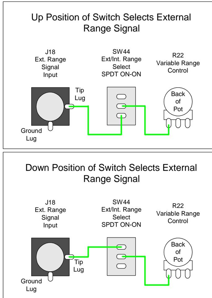
**Figure 4-16: Connection of External Range Input Option 4**
