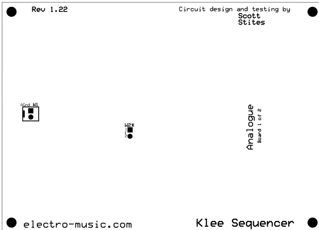
Figure 7-6: Jumper Locations on the Analogue Board
