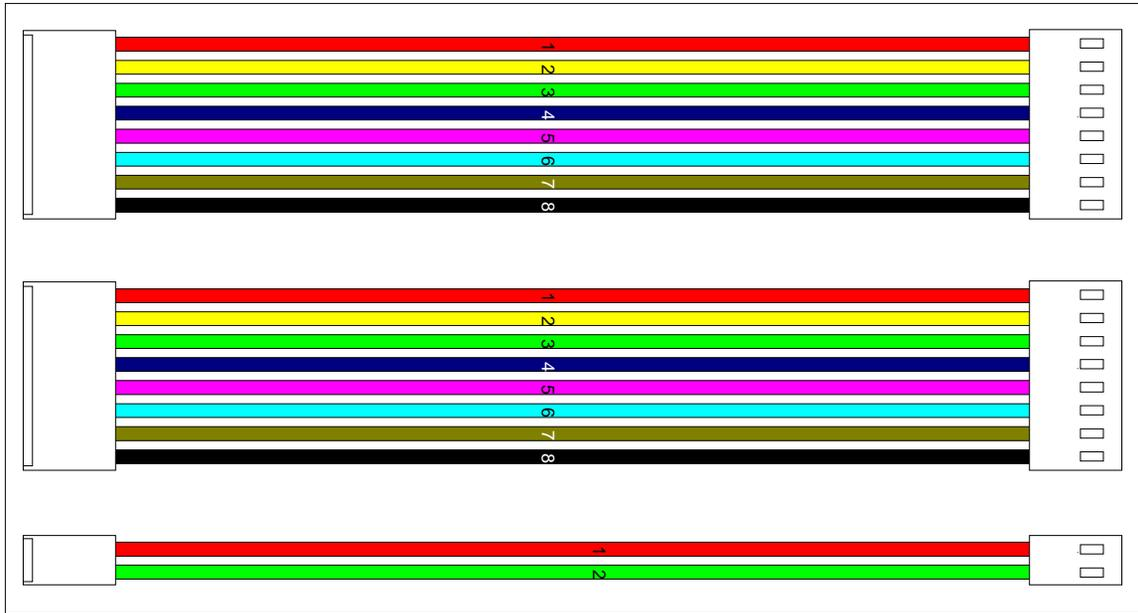
**Figure 5-5: Board Interconnect Cable Assemblies**
