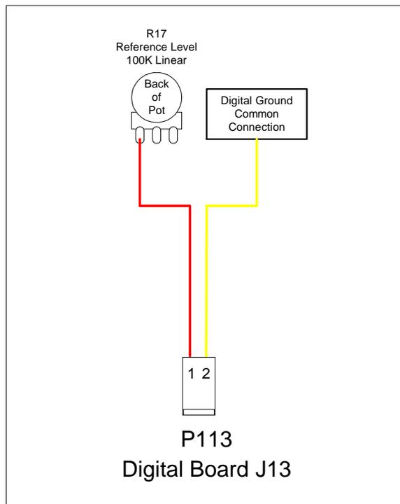
**Figure 6-19: P113 Connections**
