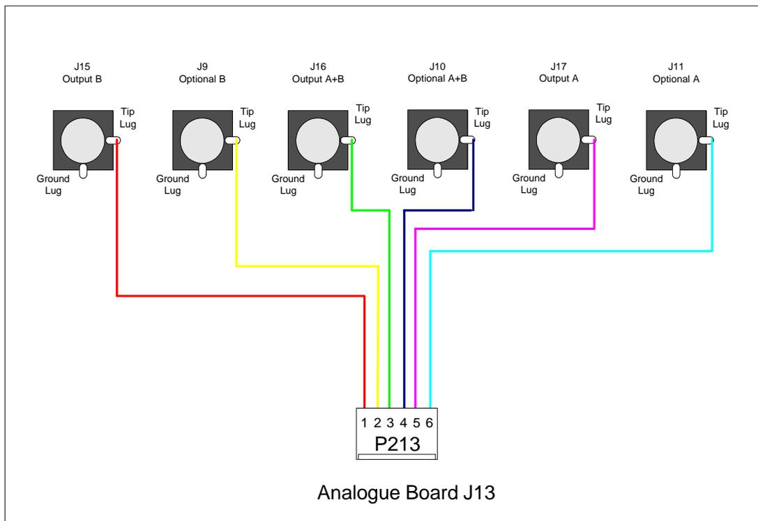
**Figure 6-17: P213 Connections**
