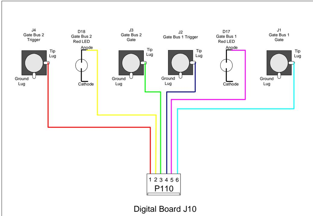
**Figure 6-14: P110 Connections**
