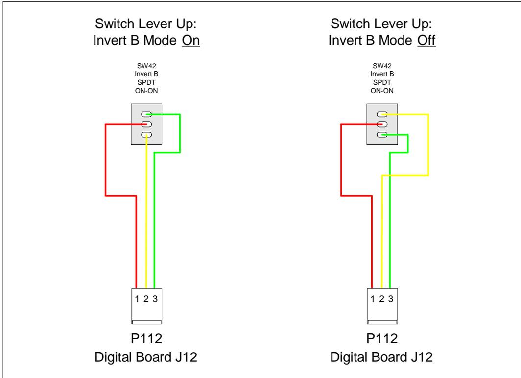
**Figure 6-18: P112 Connections**
