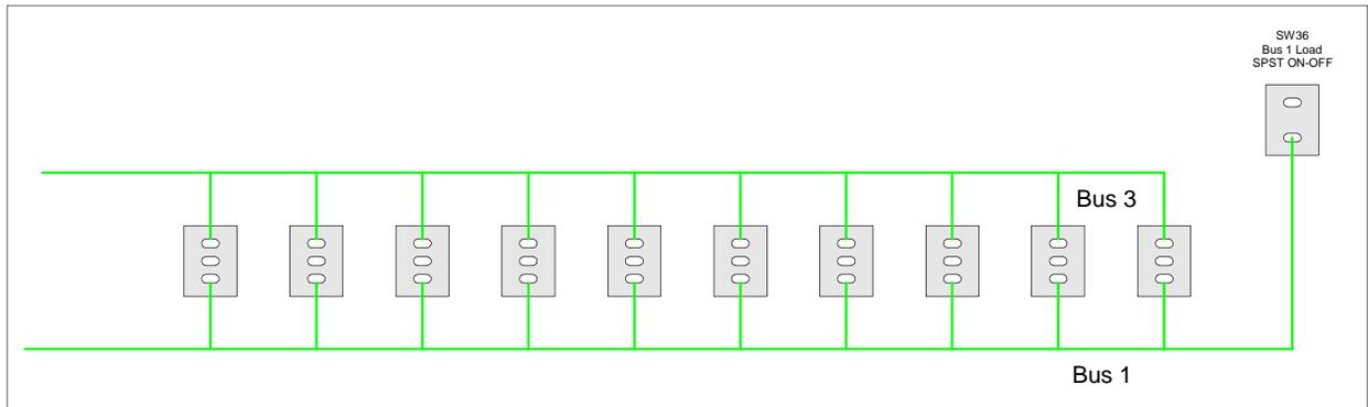
**Figure 4-9: Connecting the Bus 1 Load Switch To Bus 1**
