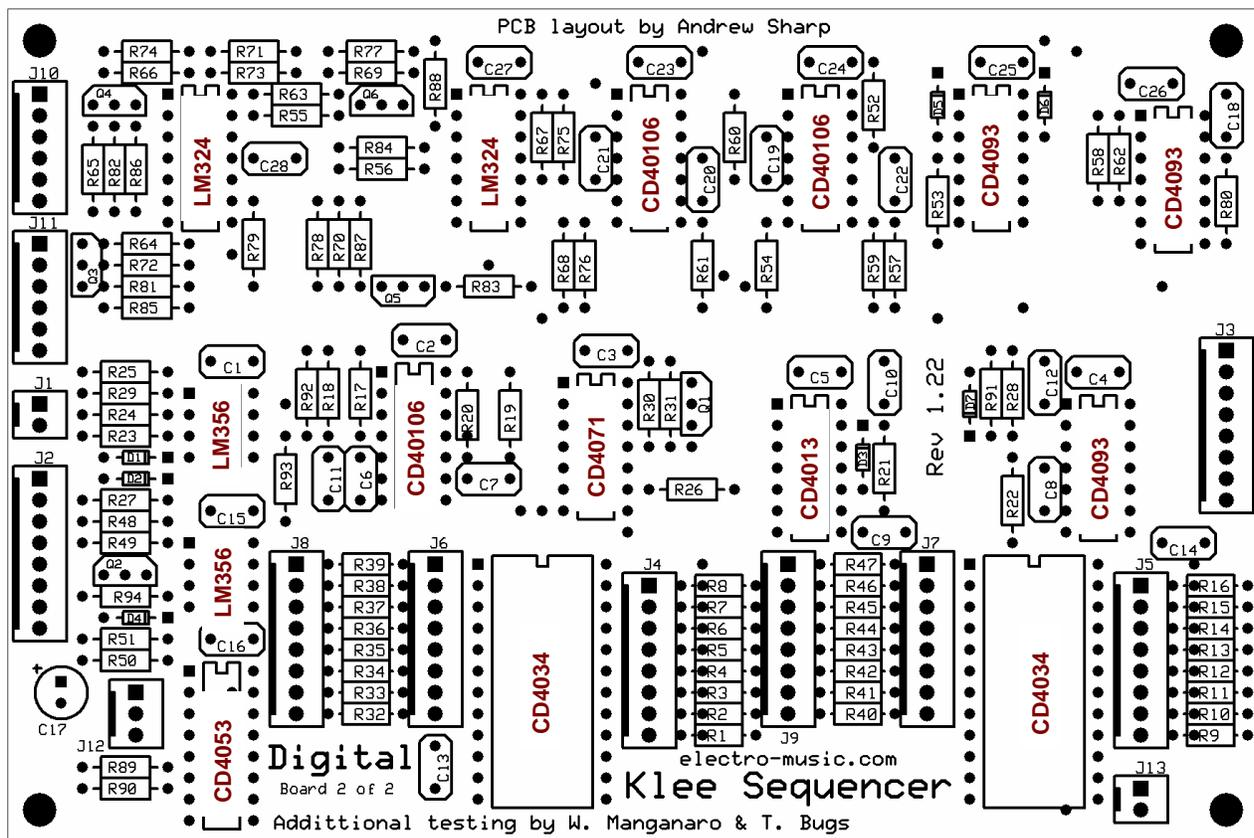
Figure 7-4: Digital Board IC Placement Guide
