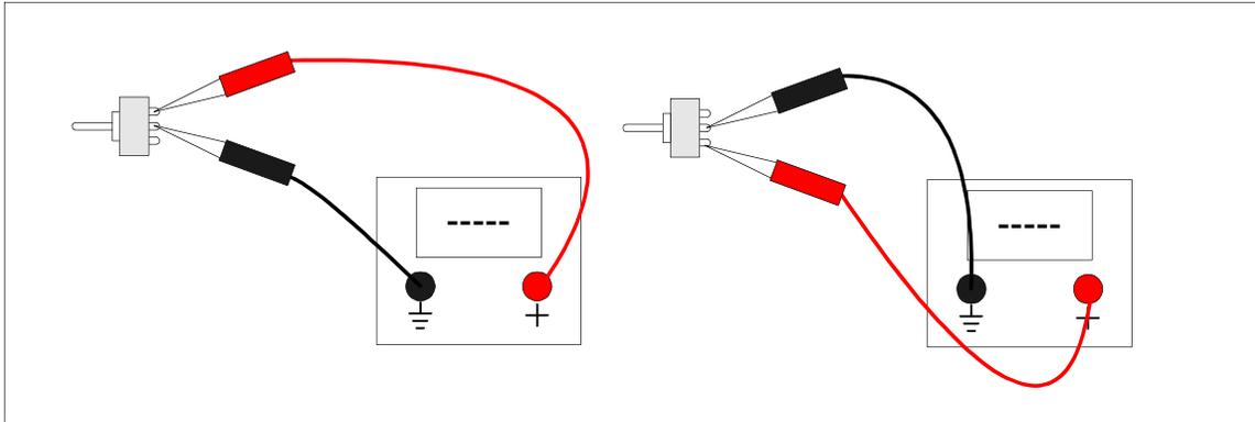
**Figure 3-2: SPDT ON-OFF-ON in the Center Position**
