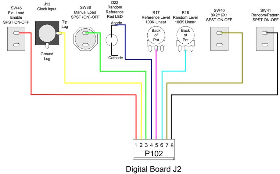
**Figure 6-11: P102 Connections**
