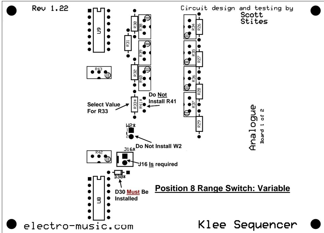
**Figure 7-8: Range Switch Position 8 Variable Range Considerations**
