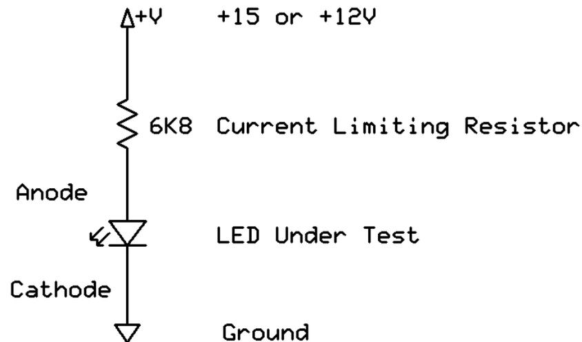
**Figure 3-5: An LED Test**
