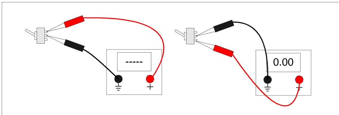
**Figure 3-1: SPDT ON-OFF-ON in the "Up" Position**
