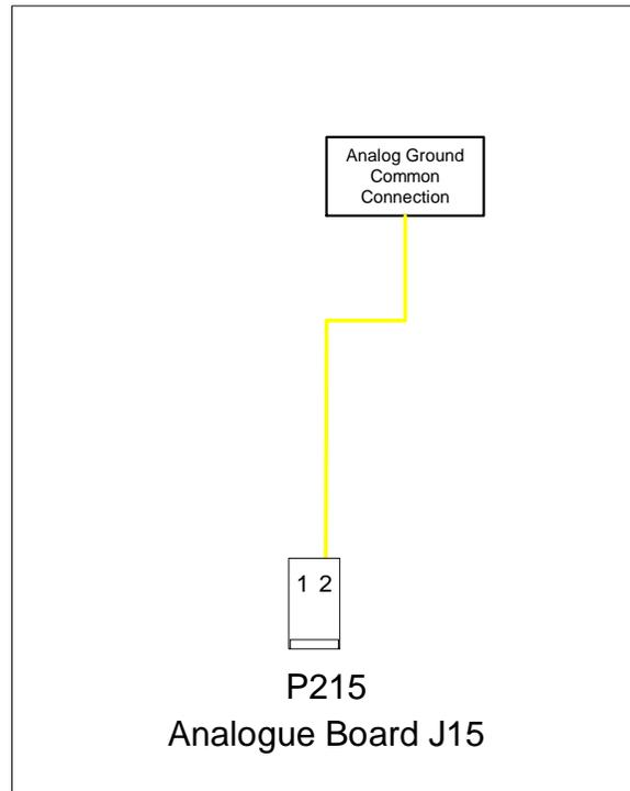
**Figure 6-20: P215 Connections**
