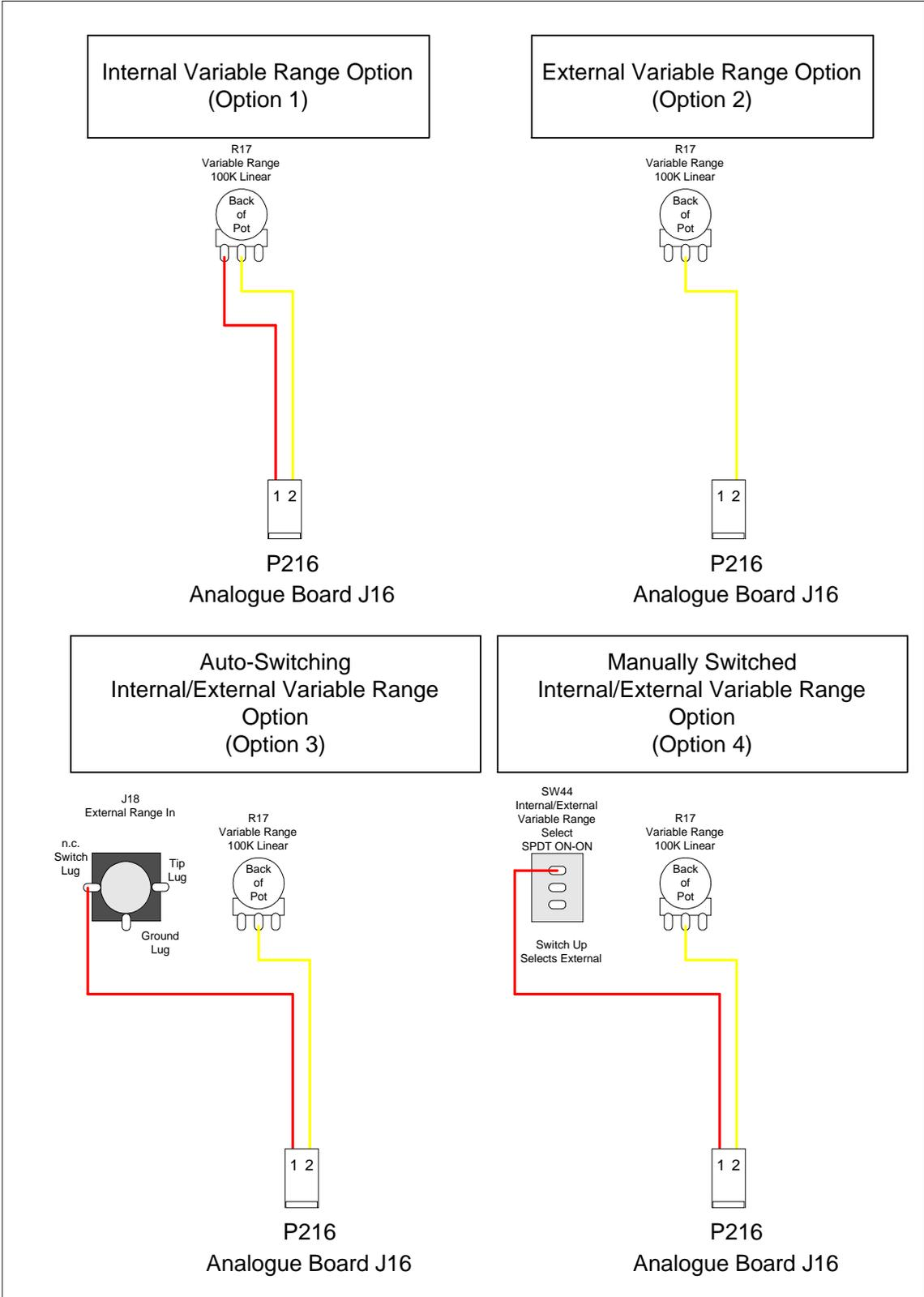
**Figure 6-21: P216 Connections (Optional)**
