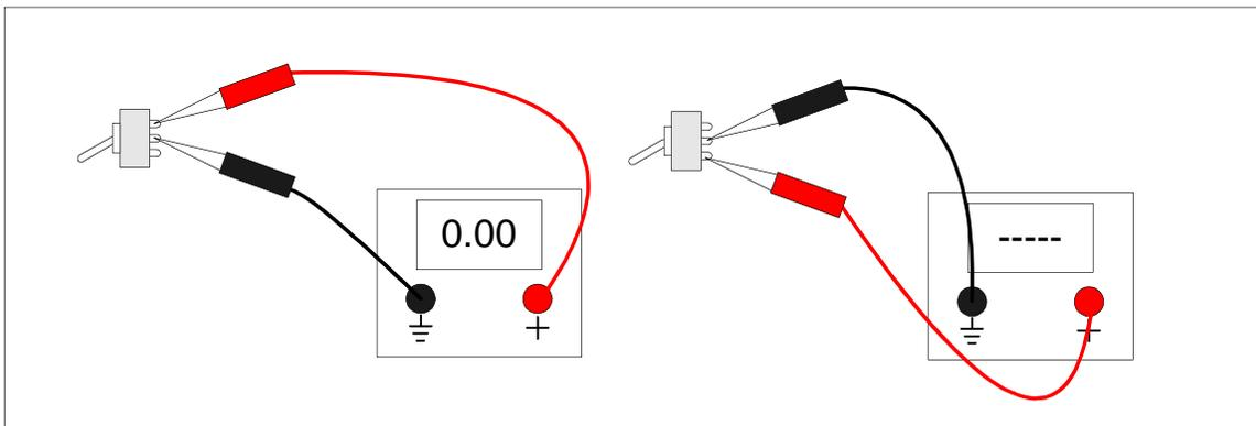
**Figure 3-3: SPDT ON-OFF-ON in the “Down” position**
