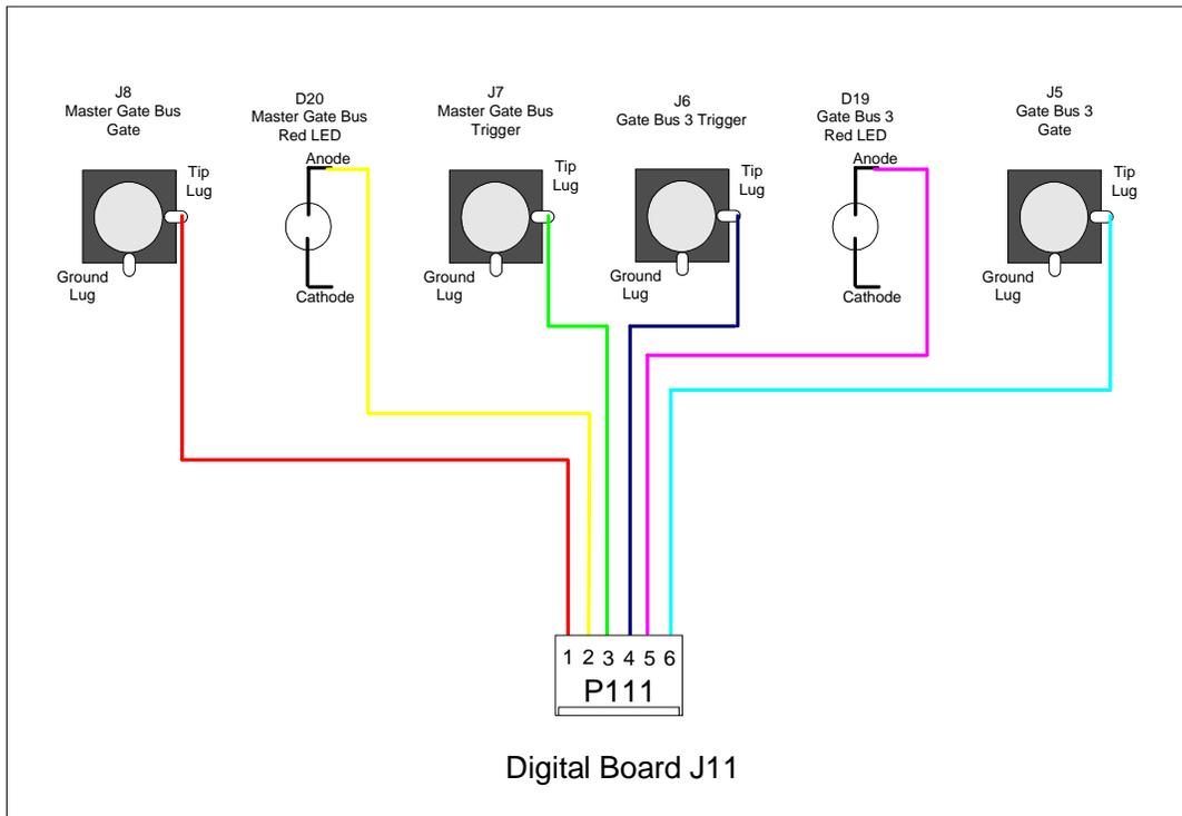
**Figure 6-15: P111 Connections**
