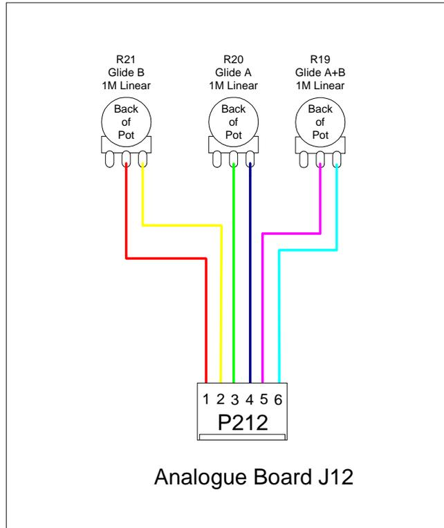
**Figure 6-16: P212 Connections**
