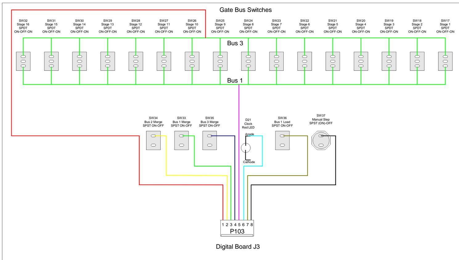
**Figure 6-13: P103 Connections**
