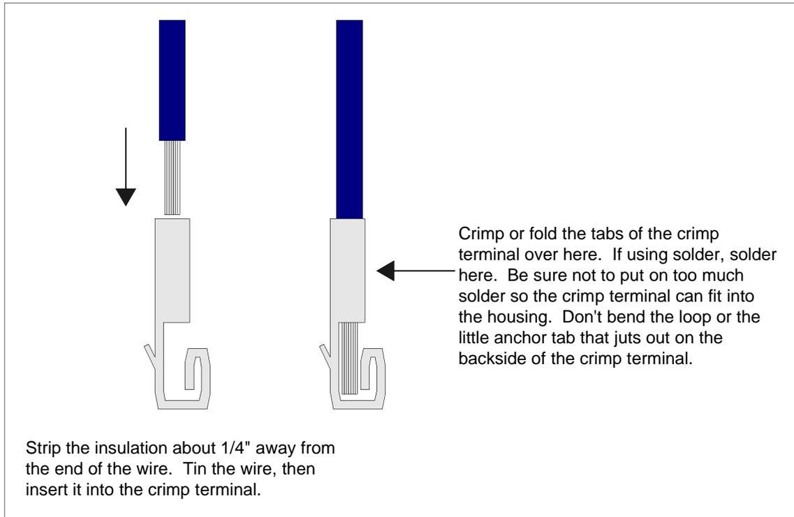
**Figure 5-2: Putting the Crimp Terminals on Wires**
