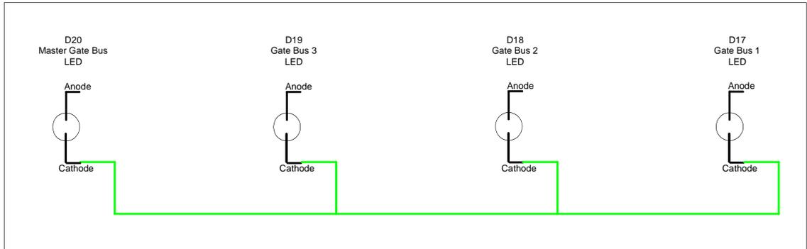
**Figure 4-3: Strap Wiring Digital Ground to the Gate Bus LEDs**
