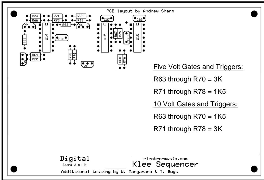
**Figure 7-3: Standard Gate Bus Resistor Locations and Values**
