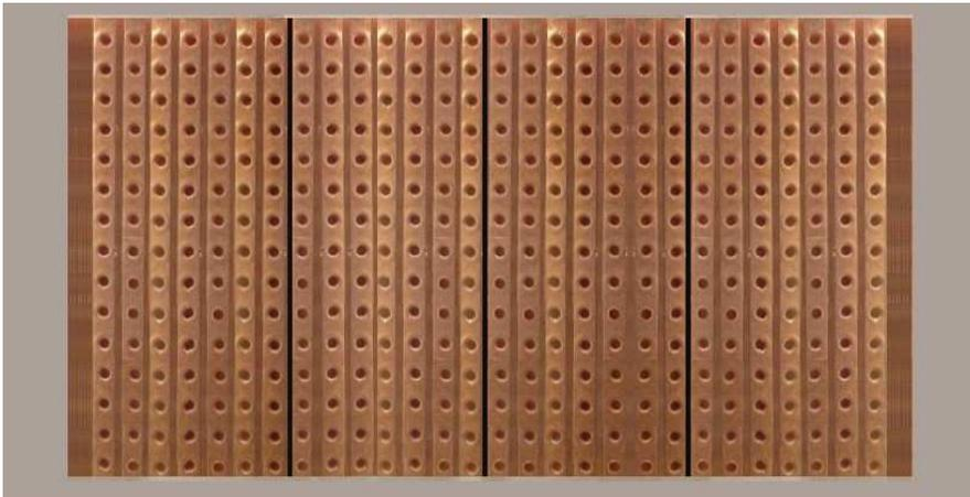
3. With a sharp hobby knife, cut the tracks as shown below to separate parts of them. You may wish to only cut the first module's tracks at this point in time; if you build it and find you made a mistake, you can correct it when you cut the other modules, once the first one is tested and working properly. When finished, turn the board over again to the component side.
