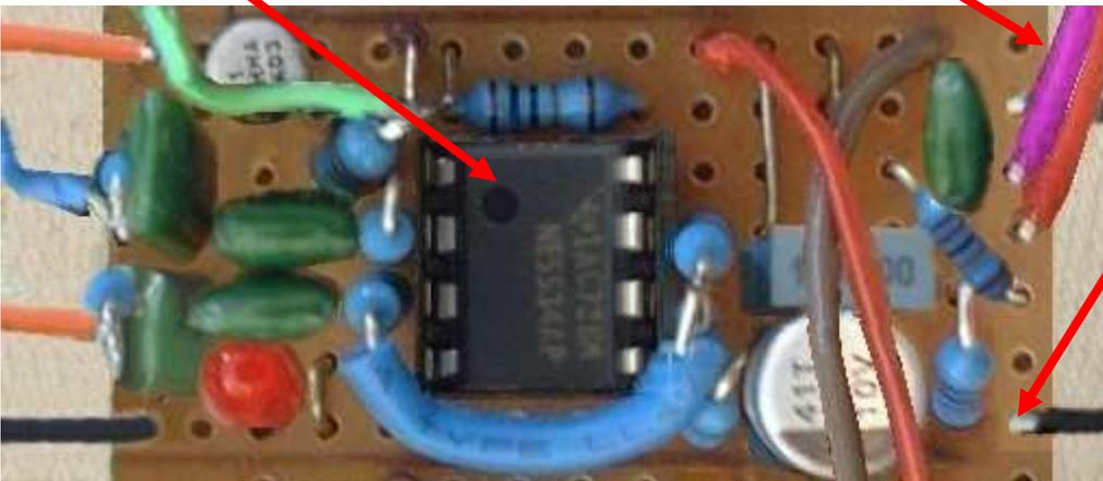
Solder a 20cm **black wire** in the hole in the board as shown here. This is the **0V ground** power lead for the circuit while it is being tested.
