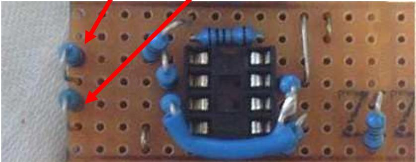
9. Solder a 20cm length of **blue** and **green** wires to the tops of the 2 resistors shown. These 2 leads go to the terminals of the 10k resonance pot (shown later).
