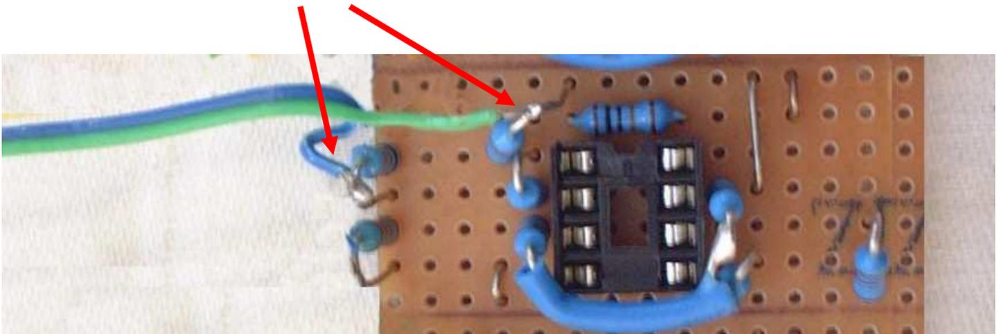
10. Solder a 20cm length of **red** and **brown** wires into the holes in the board as shown. These 2 leads go to the terminals of the 100k cutoff pot.
