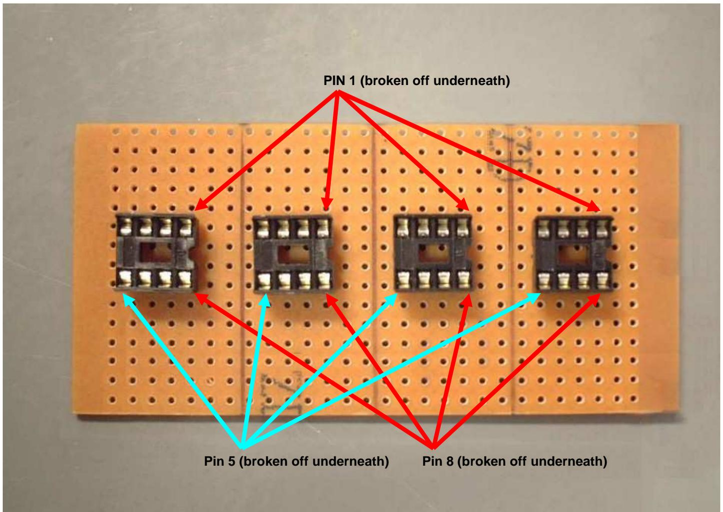
From now on, only build ONE module at a time – complete the first one, then test it to make sure it works. Then move on to the next one, then test it, etc. The board very quickly becomes crowded, and it is easy to duplicate mistakes when building the board all at once.
