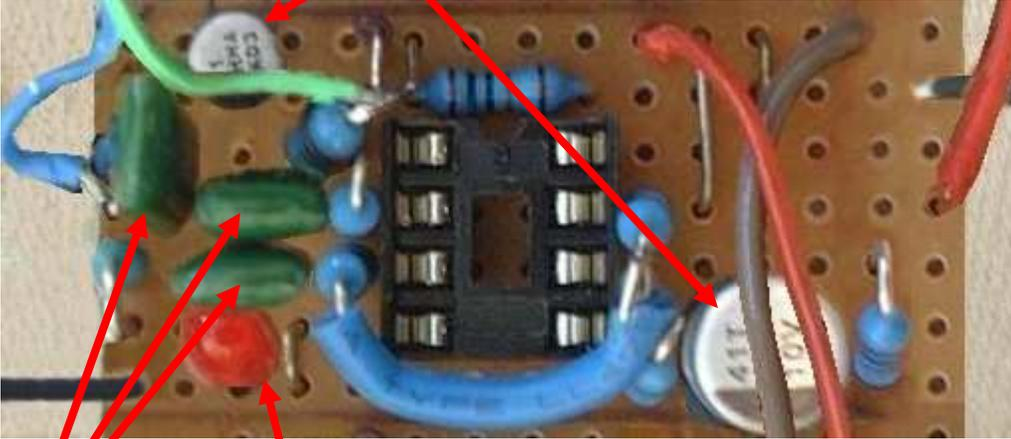
Solder in the LED, noting the correct orientation. The flat side of the base indicates the negative terminal (to the bottom of the page).
