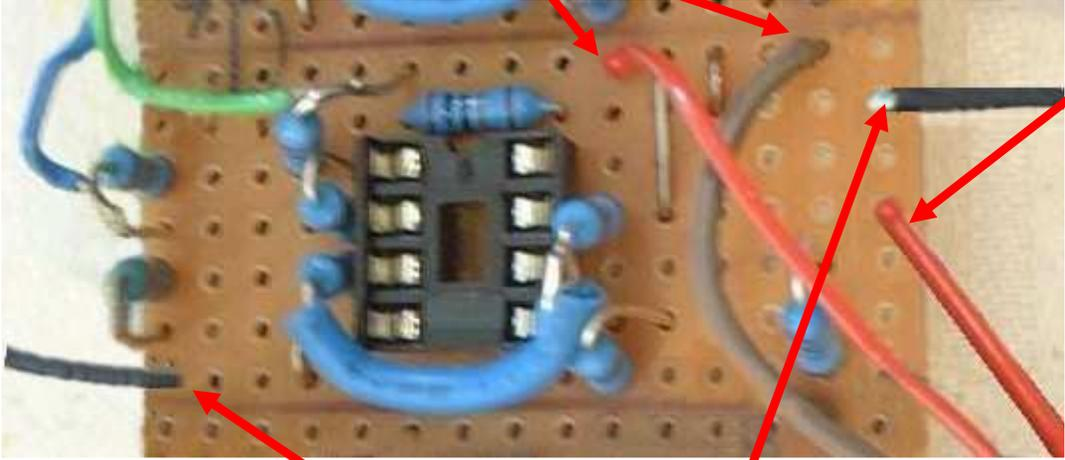
Solder a 20cm **red wire** in the hole in the board as shown. This is the 7.5V DC power lead for the circuit
