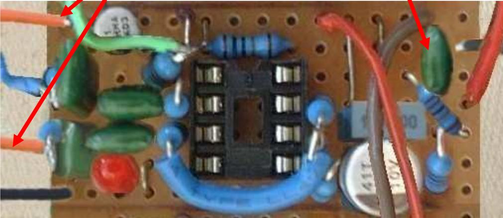
16. Insert the NE5534AN op-amp in its socket, taking note of the orientation of the chip. The dot goes to the top of the page, where the cut-out in the socket is. Solder a 20cm **purple wire** to the board here for the audio out.
