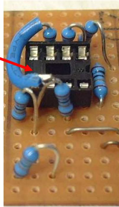
8. Solder in the 1k resistor and 470k resistor.
