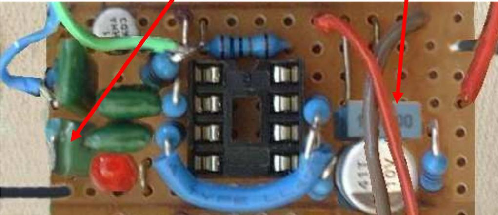
14. Solder in the 22k resistor as shown.
