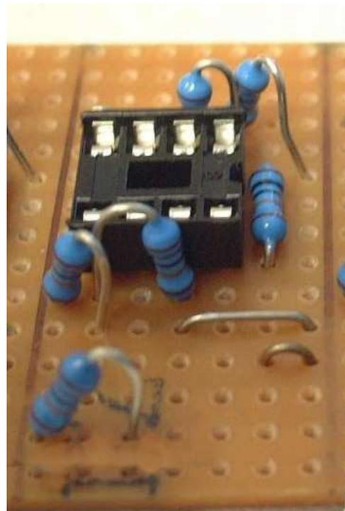
7. Solder in the 1M resistor in place.
