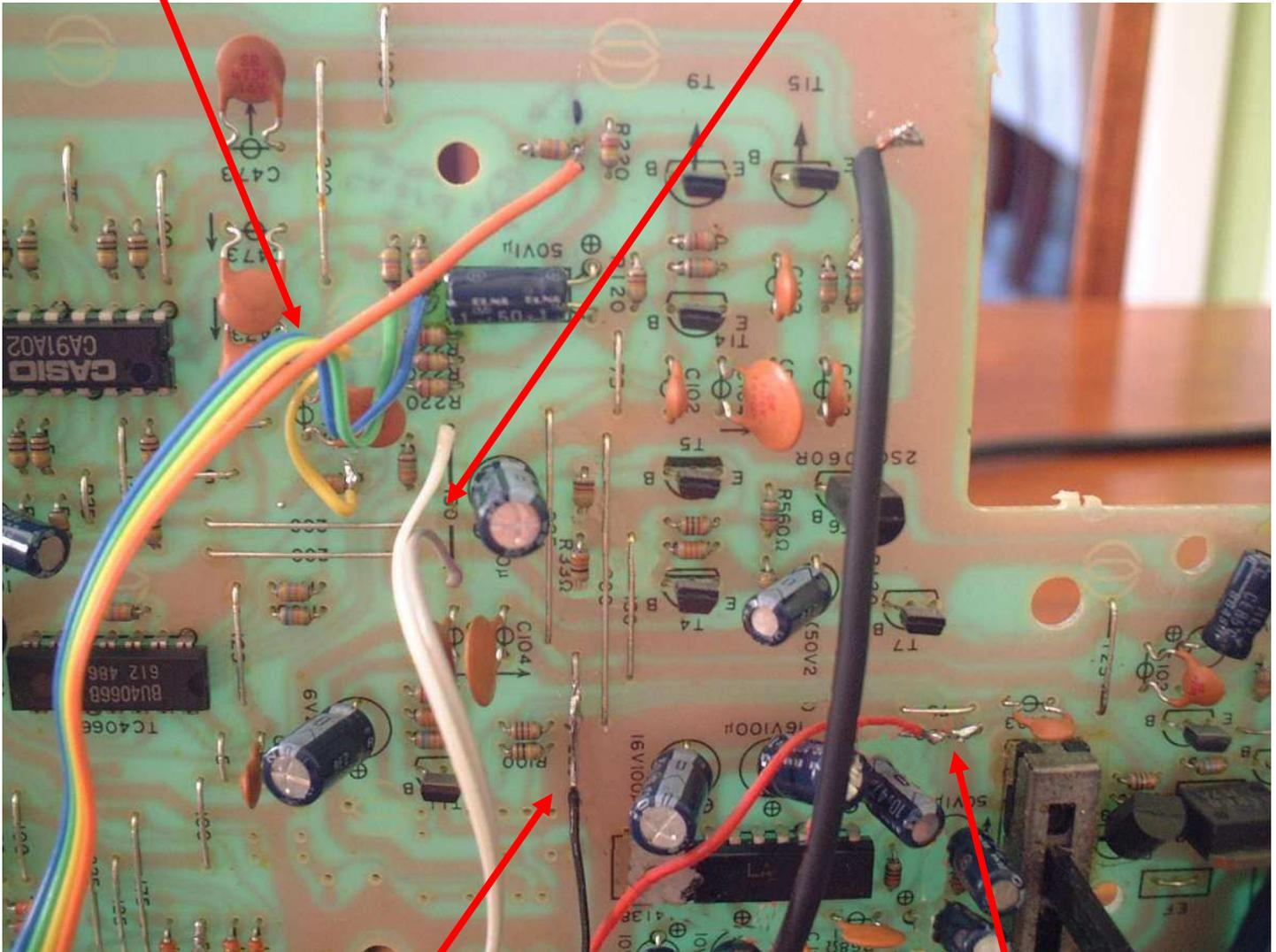
OV ground wire (black) from the **PHAT PHILTER BANK** board. It solders to this link on the SK board.
