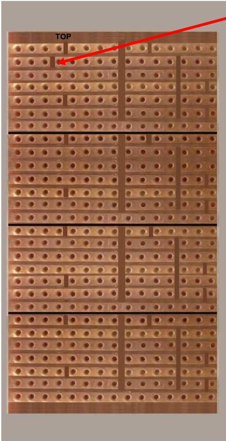
Note that this cut here is only done in the **FIRST** module – do not cut it in the other modules (although it will not cause any problems if you do – this track is unused in the other modules and will not affect the circuit)
