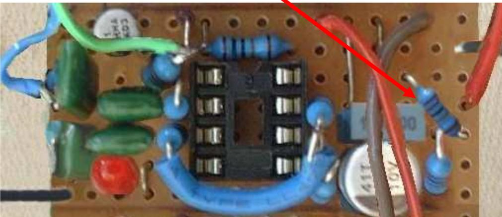
15. Solder two 20cm lengths of **orange wire** to the points below. The top one goes into a hole in the board. The lower one solders to the leg of the 470k resistor. Solder in the 0.022uF greencap capacitor. Either way will work.
