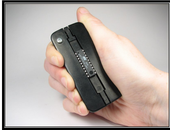
Figure 16 DIP LEAD FORMER
