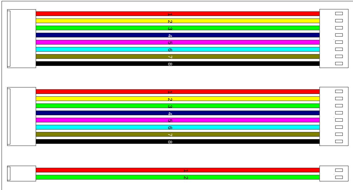
Figure 5-5: Board Interconnect Cable Assemblies
