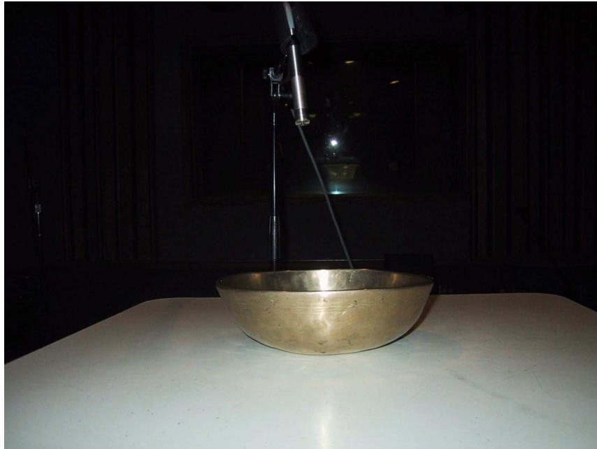
Figure 5.20: Position of the microphone used to record the impulse responses of the Tibetan bowl.
