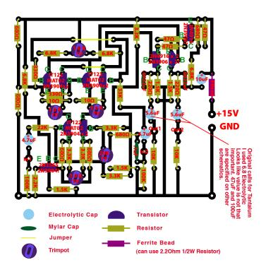
Buchla 111 Ring Mod PCB Tested and verified on 7/31/09
