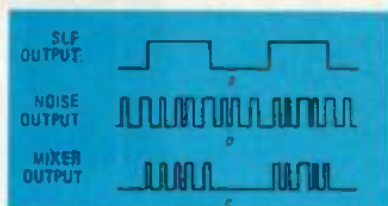
FIG. 2—THE MIXER combines the SLF output, shown in a, and a noise signal, shown in b, to produce the output shown in c.
