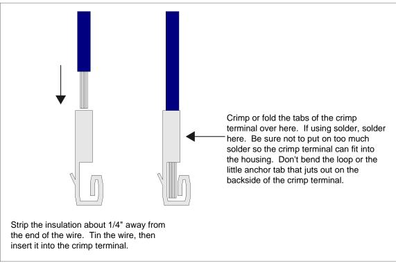
**Figure 5-2: Putting the Crimp Terminals on Wires**
