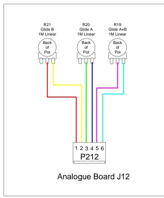
Figure 6-16: P212 Connections
