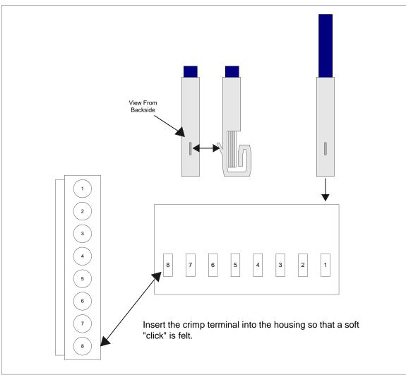
**Figure 5-4: Inserting Crimp Terminals Into the Housing**
