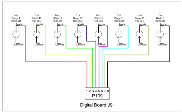
Figure 6-10: P109 Pattern LED Connections
