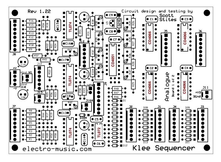
Figure 7-11: Analogue Board IC Placement Guide
