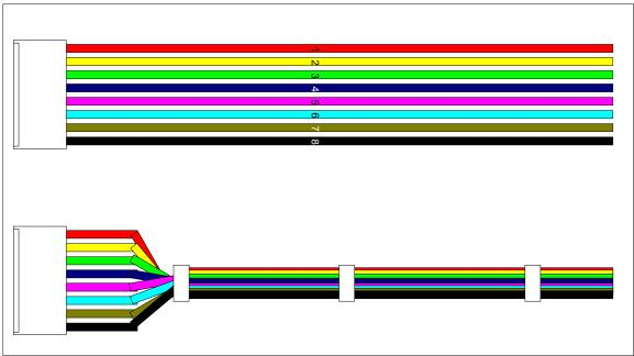
Figure 5-5: Assembled Cables
