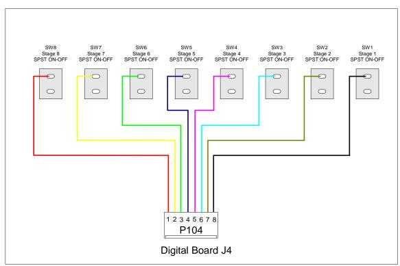
Figure 6-3: P104 Pattern Switch Connections
