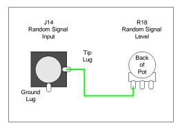
Figure 4-10: Wiring the Random Input to the Random Level Pot
