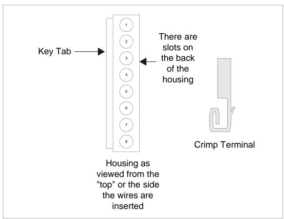
Figure 5-1: Housing and Crimp Terminal – A Graphic Anatomy
