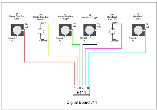
Figure 6-15: P111 Connections
