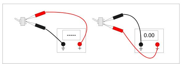
Figure 3-1: SPDT ON-OFF-ON in the "Up" Position
