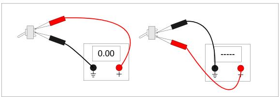
Figure 3-3: SPDT ON-OFF-ON in the "Down" position
