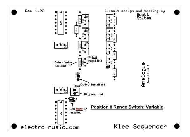
Figure 7-8: Range Switch Position 8 Variable Range Considerations
