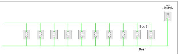
Figure 4-9: Connecting the Bus 1 Load Switch To Bus 1
