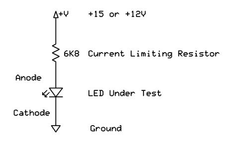
Figure 3-5: An LED Test
