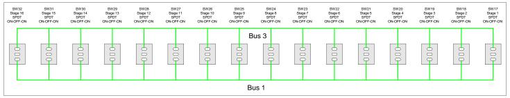
Figure 4-8: Strap Wired Gate Bus Switches – Switch Up Selects Gate Bus 1
