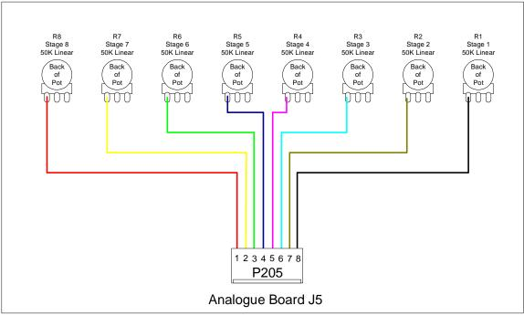
Figure 6-5: P205 Programming Pot Connections
