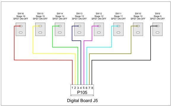
Figure 6-4: P105 Pattern Switch Connections
