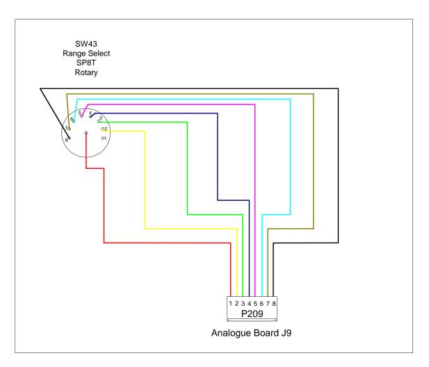
Figure 6-12: P209 Rotary Switch Connections
