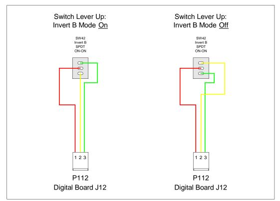
Figure 6-18: P112 Connections
