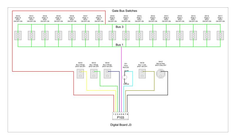
Figure 6-13: P103 Connections
