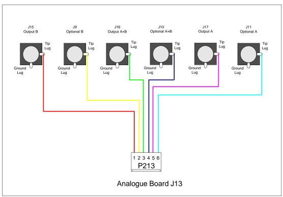
Figure 6-17: P213 Connections
