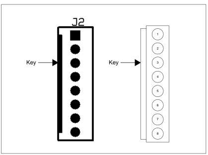
Figure 7-2: Orientation of PCB Header Connectors
