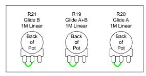
Figure 4-12: Wiring the Unused Lug to the Center Tap of the Glide Pots
