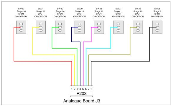
Figure 6-2: P203 Gate Bus Switch Connections
