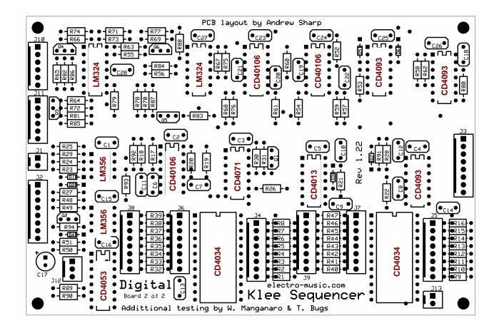
Figure 7-4: Digital Board IC Placement Guide
