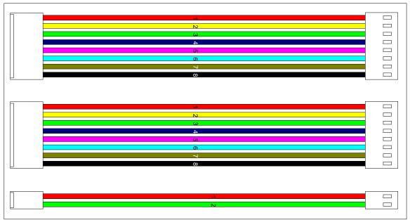
Figure 5-5: Board Interconnect Cable Assemblies
