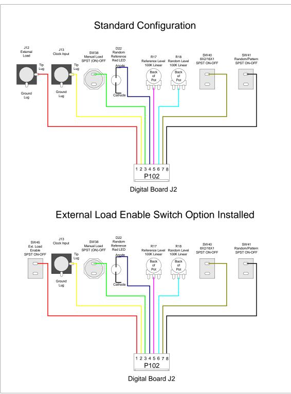
Figure 6-11: P102 Connections
