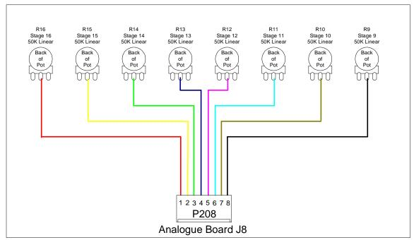
Figure 6-8: P208 Programming Pot Connections
