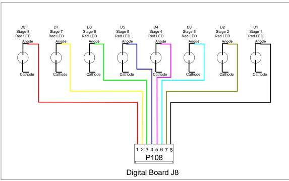
Figure 6-9: P108 Pattern LED Connections
