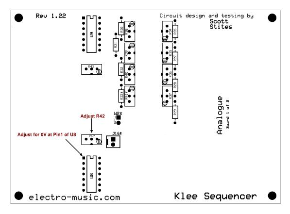
Figure 10-1: Register A Offset Zero Calibration
