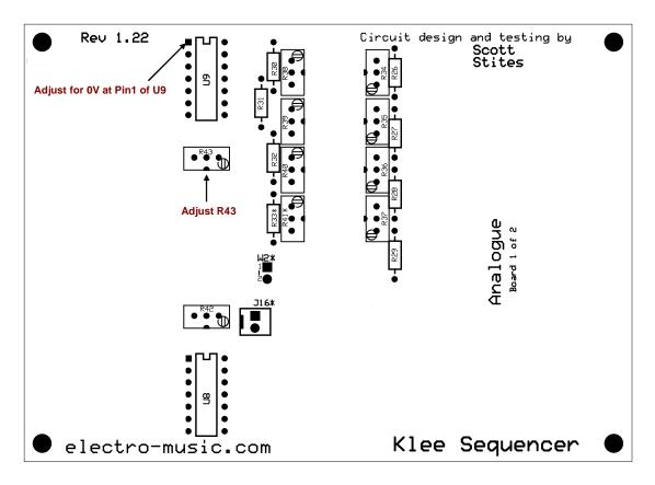
Figure 10-2: Register A Offset Zero Calibration
