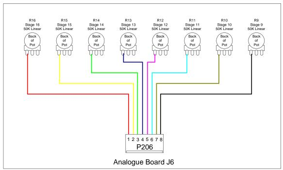
Figure 6-6: P206 Programming Pot Connections
