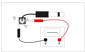
Figure 3-10: Cable Inserted – N.C. Lug Open
