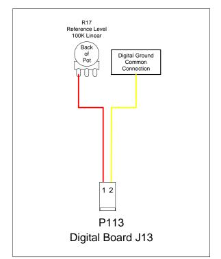
Figure 6-19: P113 Connections
