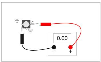
Figure 3-9: No Cable Attached – N.C. Lug Closed
