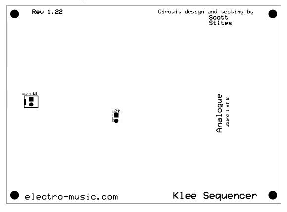
Figure 7-6: Jumper Locations on the Analogue Board
