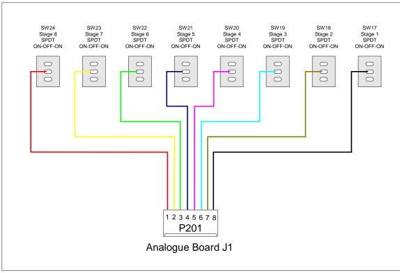
Figure 6-1: P201 Gate Bus Switch Connections
