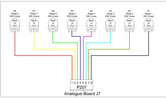
Figure 6-7: P207 Programming Pot Connections
