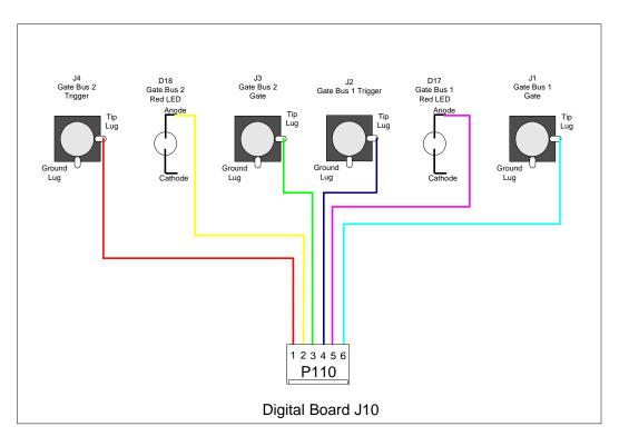
Figure 6-14: P110 Connections
