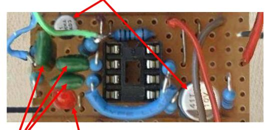
Solder in the LED, noting the correct orientation. The flat side of the base indicates the negative terminal (to the bottom of the page).
