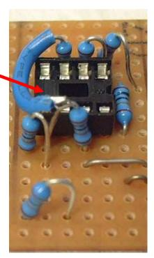
8. Solder in the 1k resistor and 470k resistor.
