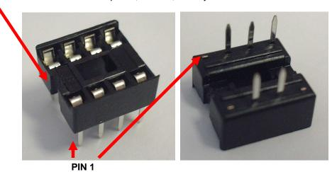
Put the IC in position on the board as shown, and solder in place.
