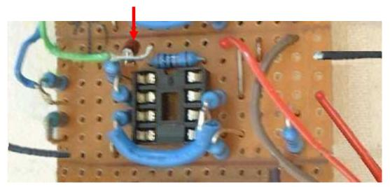
12. Solder in the 1uF and 47uF electrolytic capacitors. Make sure they are orientated the correct way (the black end is the negative terminal).
