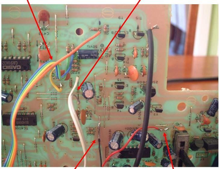
OV ground wire (black) from the **PHAT PHILTER BANK** board. It solders to this link on the SK board.
