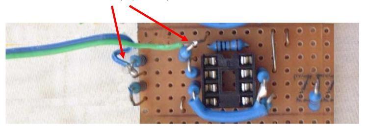
10. Solder a 20cm length of **red** and **brown** wires into the holes in the board as shown. These 2 leads go to the terminals of the 100k cutoff pot.
