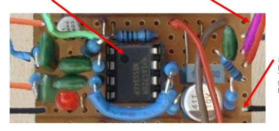
Solder a 20cm **black wire** in the hole in the board as shown here. This is the **0V ground** power lead for the circuit while it is being tested.
