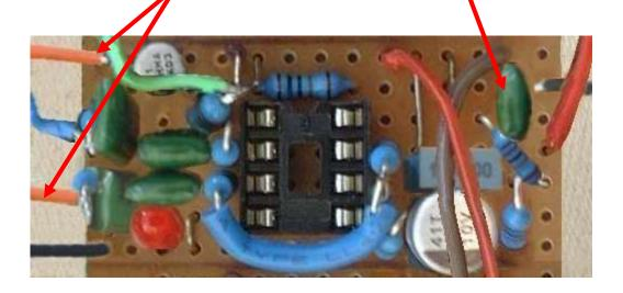
16. Insert the NE5534AN op-amp in its socket, taking note of the orientation of the chip. The dot goes to the top of the page, where the cut-out in the socket is. Solder a 20cm purple wire to the board here for the audio out.
