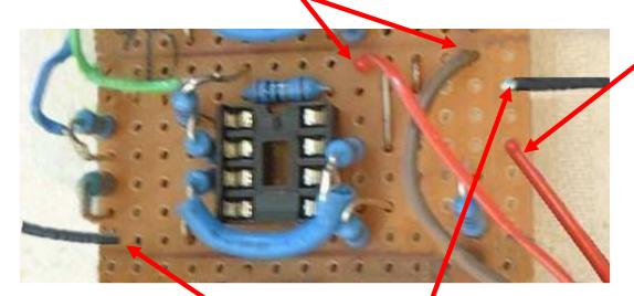
Solder a 20cm red wire in the hole in the board as shown. This is the 7.5V DC power lead for the circuit
