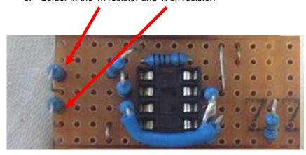
9. Solder a 20cm length of **blue** and **green** wires to the tops of the 2 resistors shown. These 2 leads go to the terminals of the 10k resonance pot (shown later).
