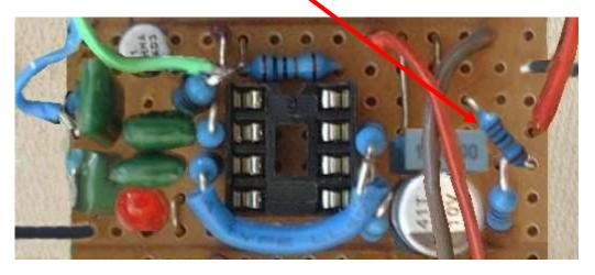
15. Solder two 20cm lengths of **orange wire** to the points below. The top one goes into a hole in the board. The lower one solders to the leg of the 470k resistor. Solder in the 0.022uF greencap capacitor. Either way will work.
