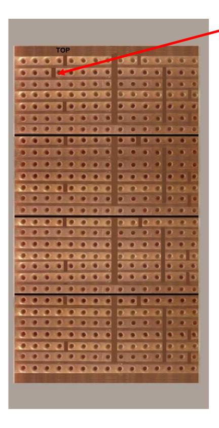
Note that this cut here is only done in the **FIRST** module – do not cut it in the other modules (although it will not cause any problems if you do – this track is unused in the other modules and will not affect the circuit) 4. Take an 8-pin IC socket, and orientate the notch in one end to the top of the page. This is the IC orientation notch. Break off pins 1, 5 and 8, so they do not connect with the circuit board.
