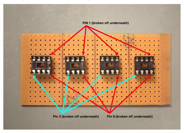
From now on, only build ONE module at a time – complete the first one, then test it to make sure it works. Then move on to the next one, then test it, etc. The board very quickly becomes crowded, and it is easy to duplicate mistakes when building the board all at once.
