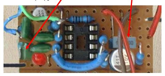
14. Solder in the 22k resistor as shown.
