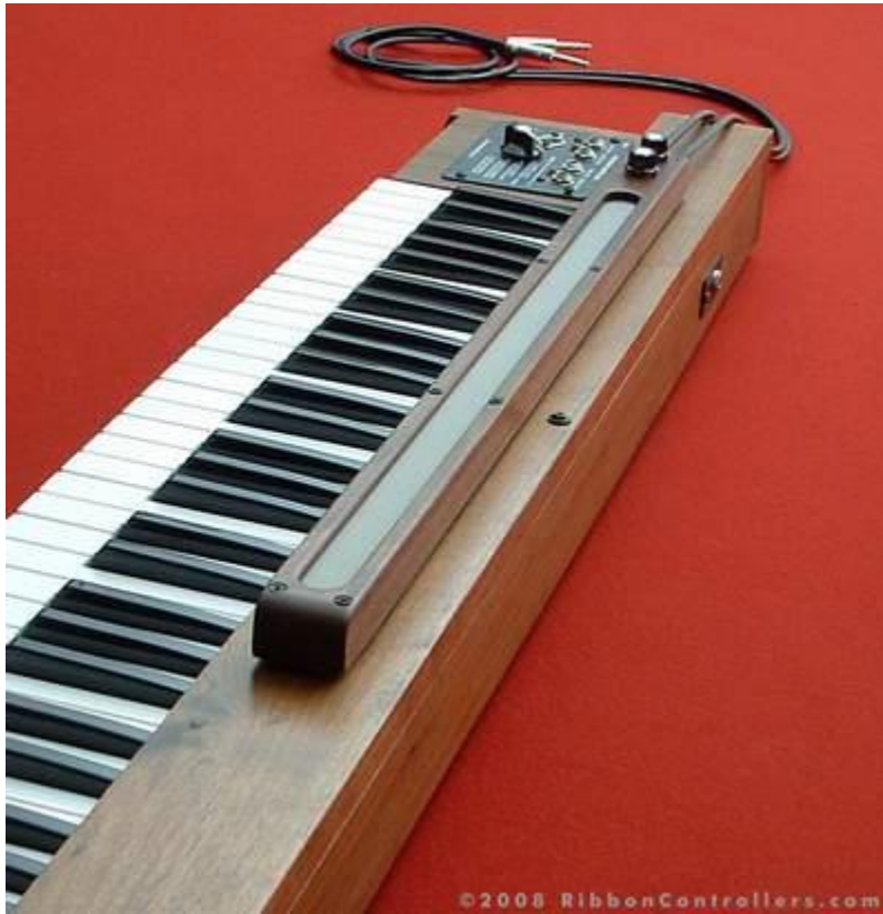
Figure 1-3: Example of a Pre-Manufactured Ribbon Assembly
