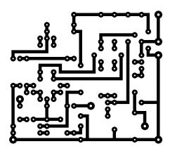
Originally this design used 2N3565 transistors, and an IT122 matched pair for pair on the left. 2N3904s or any standard NPN will probably work for all of them. Can also try MAT02, etc... as a sub for the matched pair.
