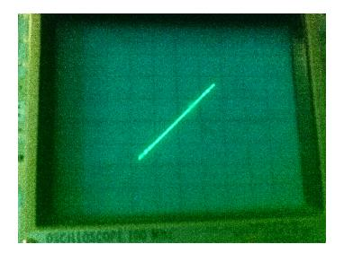
The photo below shows our linear CMOS gate's transfer function. It looks just like a digital CMOS transfer function with it's flat horizontal regions at the high and low values of input signal, however there is a region in the middle that has a slope of minus ten. The circuit will self-bias at the middle of that slope and wiggle up and down in response to small changes in the input signal wiggling.
