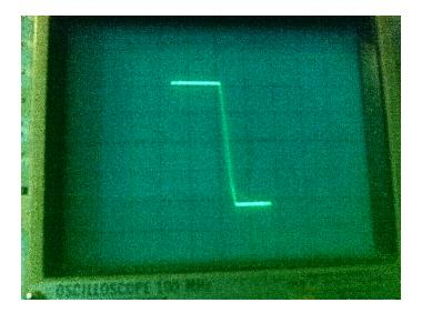
The plot below shows the transfer function of the linear CMOS gate when the gain is set to minus one. We have our slope of negative one, however the circuit is self-oscillating which makes an undesired audio signal. We don't want the self-oscillation so we use larger gains to stop that from happening.
