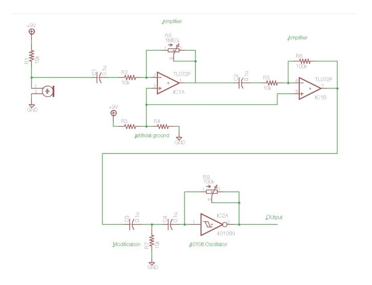
The microphone itself works like a variable resistor of about 10k Ohms resistance, so we put it in a voltage divider with a 10k resistor to power it. It sends out a very weak signal so we have to amplify it by about 1000 times. The first amplifier has a gain of -100 and the second a gain of -10, for a total gain of 1000. The way to calculate the gain of an inverting amplifier is to divide the feedback resistance by the input resistance and multiply by minus one.
