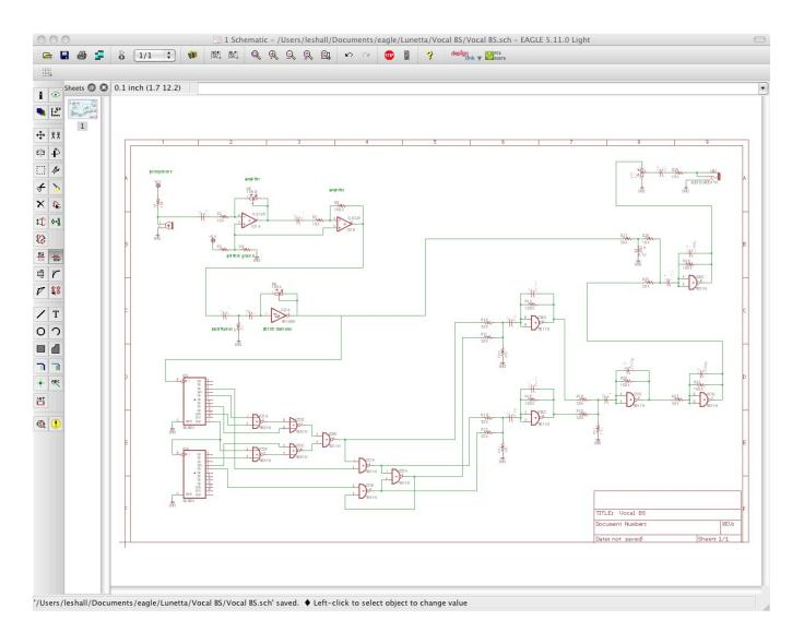
That's a lot to discuss, so we are fortunate that we have no time limit on this week's show. Let's begin with the power supply starve pot. It consists of a 100k potentiometer hooked up in series with the power supply and with a 10k resistor in parallel with it. The pot is hooked up like a rheostat, using one end and the center tap only, forming a variable resistor. The idea behind this addition is to add an interesting musical feature: supply starving.
