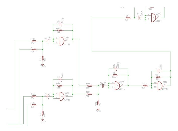
We have two input gates with two inputs each, a second gate combining the outputs of the first two, and finally a gain stage to boost the audio levels. This is another circuit that I recently designed for the purpose of creating this week's show.
