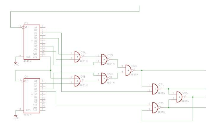
The logic is just a randomly connected set of whatever gates you have on hand and you can experiment with different wiring to get different sounds. Note also that on the lower right I accidentally created state information by using logic feedback. This was unintentional but it serves to create more variety in the sound, so feel free to do this.
