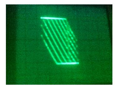
The plot is very nice for music applications because it has smoothly varying mid-level signals and sharply changing upper and lower signals. In effect, it mixes the digital inputs to create analog levels. To really make good sound, however, we need a few layers of such a circuit. I got away using only two layers but more would have been better.
