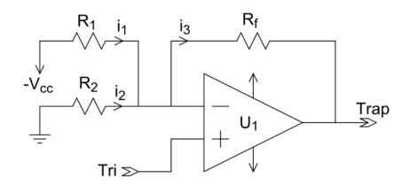
In an effort to understand what's going on with this circuit, I'm going to try to derive its transfer function  $\frac{Trap}{Tri}$ :
