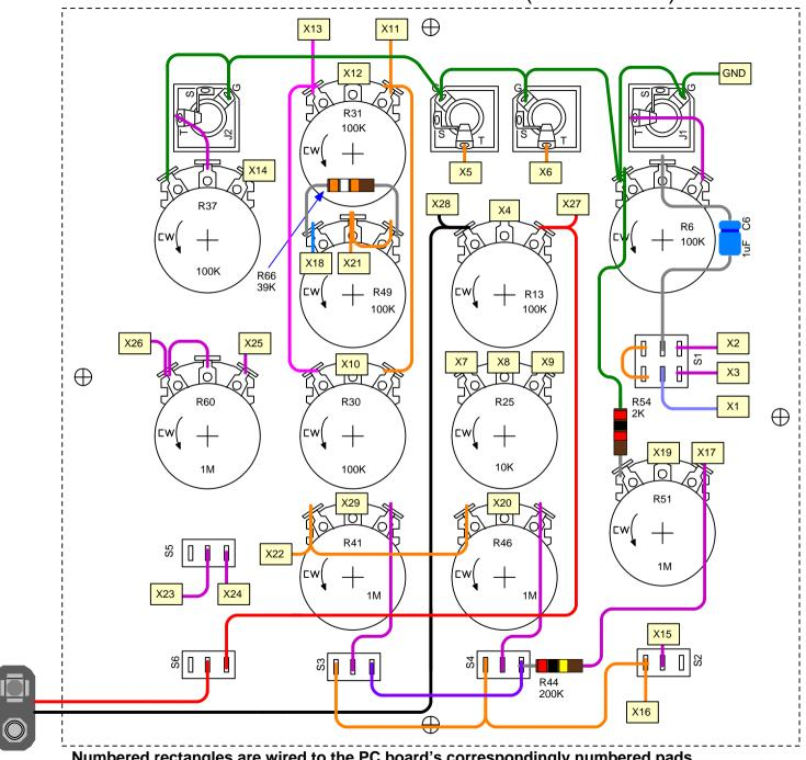
Numbered rectangles are wired to the PC board's correspondingly numbered pads.
